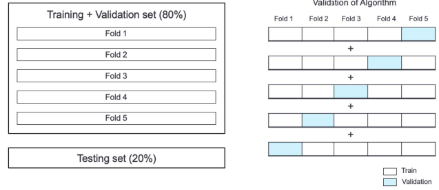
Fig. 5. Schematic of the data partition and the training of the algorithm including k -fold validation step.
